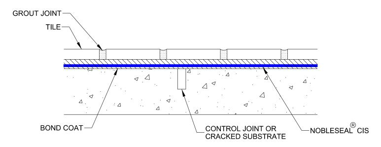
CONTROL JOINTS (CONSTRUCTION, ISOLATION, CONTRACTION)
