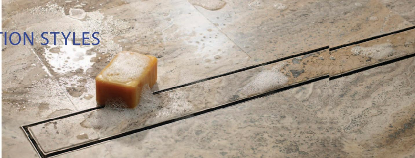
Fit and finish. Grate designs and finishes vary by manufacturer, from simple stamped plates to heavy-gauge wedge wire. Many also offer a "tile-in" version (left) that allows you to tile the top of the linear-drain grate so that it matches the rest of the shower floor. This often is the least expensive linear-drain option.
