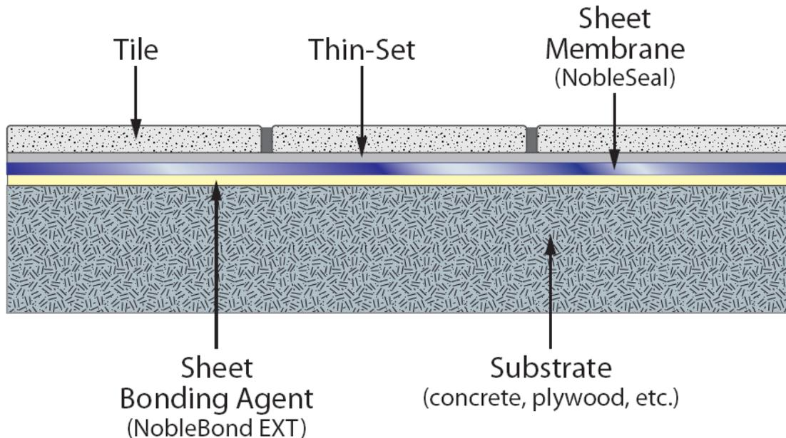
**Thin-bed methods** utilize a thin-set mortar (cement) to adhere tile to a substrate (like concrete, mortar bed, plywood, etc.). Some thin-sets are fortified with latex (polymeric or acrylic) to increase the adhesive properties and flexibility.
