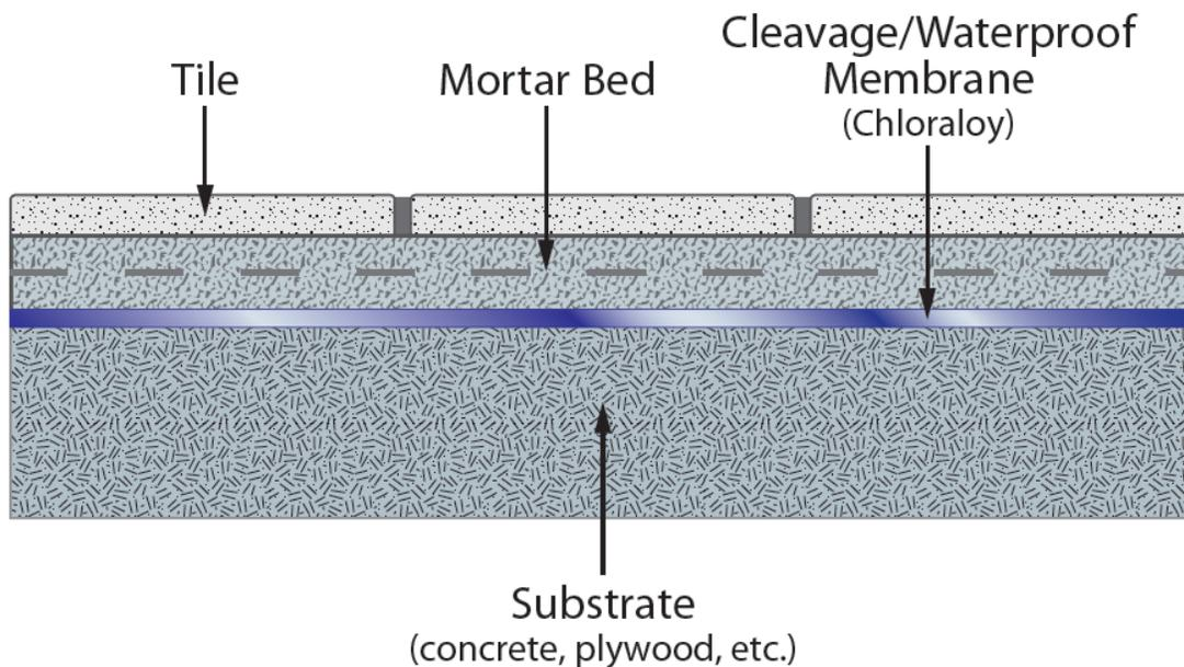
**Mortar bed methods** have been used for centuries and have proven to be dependable. They are also referred to as thick bed, full mortar bed or mud bed methods. Method involves the following:
